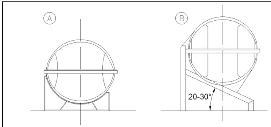
**Figure 1 – Mounting arrangements**
